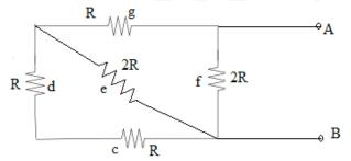
Resistors c and d are connected in series combination Thus  $R_{cd}=R+R=2R$
